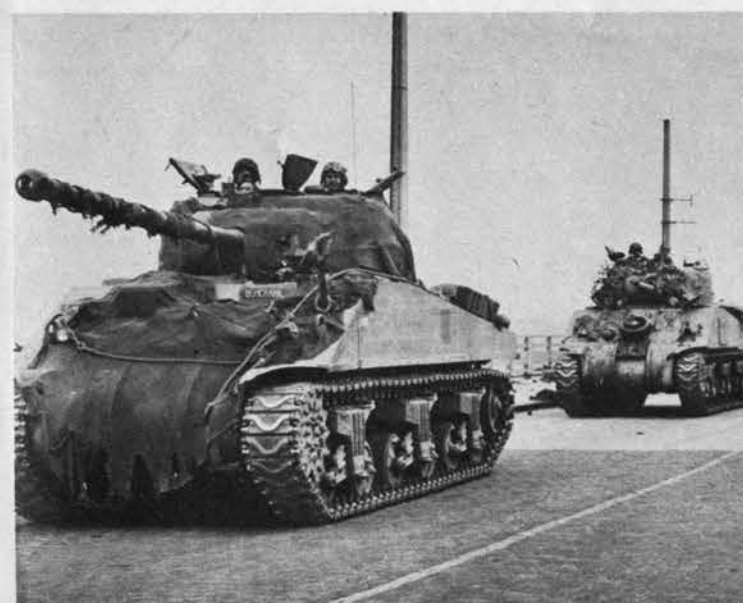
British Shermans rumble across the famous bridge at Nijmegen. Like the tank in the foreground, many of them carry as their main armament a long, high-velocity 17-pounder with a bottlelike muzzle brake.
